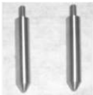
图 1 铁棒在浸入注水 MIL-PRF-5606 液压油中 4 h 后无腐蚀 Fig. 1 No corrosion occurs on iron bar after 4 h in MIL-PRF-5606 hydraulic oil with water affusion
