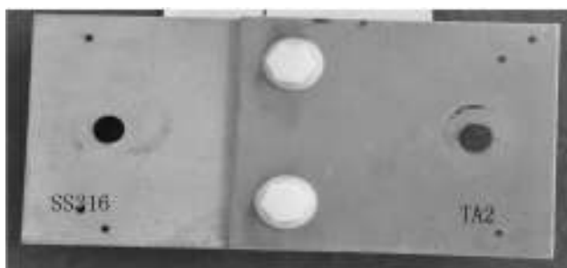
图2 深海暴露 200 d 的偶合试样 Fig. 2 The coupling sample after exposure in deep sea environment for 200 d
