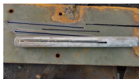
图 7 等离子切割试验效果 Fig.7 Effect of plasma cutting test
