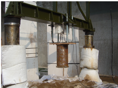
图 4 某产品的跌落试验初始状态 Fig.4 The initial state for the drop-test sample
