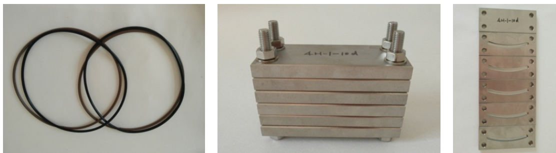
图 1 典型橡胶密封圈及试验夹具 Fig.1 Typical rubber seal ring and test fixture
