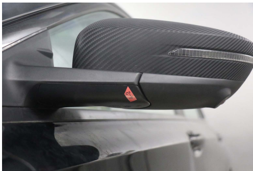
图 7 后视镜固定支架上下盖板离缝 Fig.7 Gap between the upper and lower covers of the rearview mirror fixing bracket
