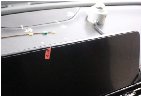
图 6 中控显示屏中框变形脱胶 Fig.6 Deformation and degumming of the central control display frame
