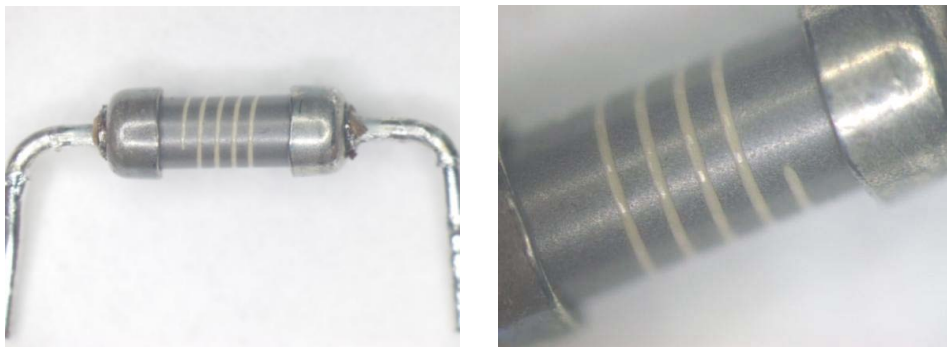
图 7 金属膜电阻典型内部形貌 Fig.7 Typical internal morphology of the metal film resistance
