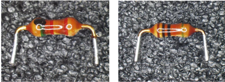
图 6 金属膜电阻典型外观形貌 Fig.6 Typical morphology of metal film resistance
