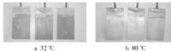
图1 不同海水温度下6061铝合金浸泡35 d后的腐蚀形貌 Fig. 1 Corrosion morphology of 6061 after 35 d immersion in different temperature seawater
