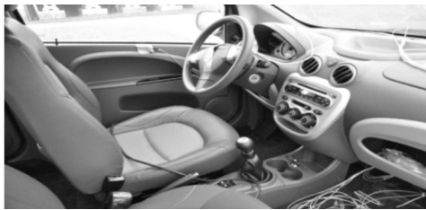
图2 整车内部温度传感器 Fig.2 Interior temperature sensors set
