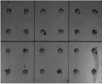
图4 未涂缓蚀剂内部结构试验件3个周期后的腐蚀情况 Fig.4 Corrosion of the interior structure samples not coated with corrosion inhibitor after three cycles of test
