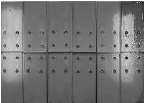
图 2 涂缓蚀剂试验件 Fig. 2 The samples coated with corrosion inhibitor
