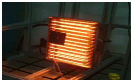
图 11 6061-T6 矩形铝板热模态试验 Fig.11 Thermal modal test of 6061-T6 rectangular aluminum plate
