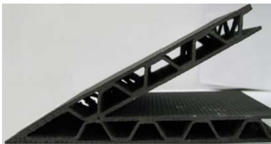
图 10 C/SiC 波纹点阵结构进气道前缘样件 Fig.10 Sample of C/SiC inlet leading edge with corrugated lattice structure
