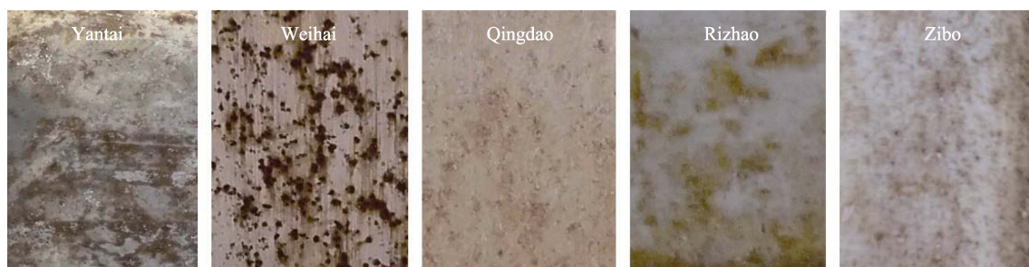
图 1 烟台、威海、青岛、日照、淄博不锈钢结构的腐蚀 Fig.1 Corrosion of stainless steel structures in Yantai, Weihai, Qingdao, Rizhao and Zibo of Shandong, China
