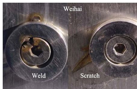
图 15 不锈钢在焊接或表面擦伤处发生腐蚀 Fig.15 Corrosion of stainless steel at welding points or surface scratches
