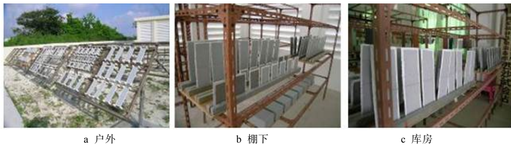
图 3 自然环境暴露试验 Fig.3 Natural environment exposure test: a) outdoor; b) under roof; c) storage room
