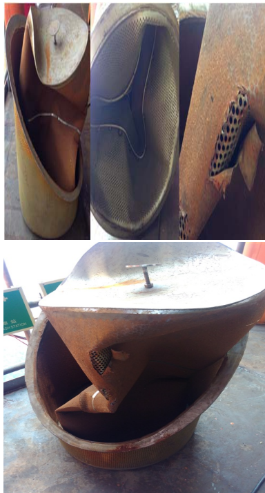
图 2 滤芯变形、腐蚀图片 Fig.2 Deformation and orrosion of filter element
