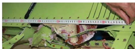
图 11 前缘舱梁仿真结果与试验结果对比 Fig.11 Comparison between simulation results and experiment resultsof leading edgeauxiliary spar
