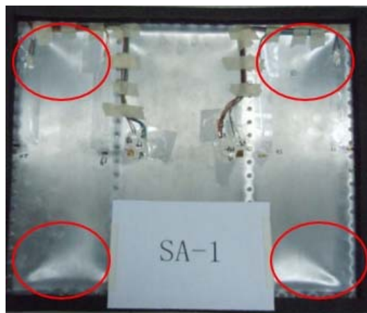
图6 声静联合试验中发生塑性变形的试验件 Fig.6 Test pieces for plastic deformation in combined acoustic and static test
