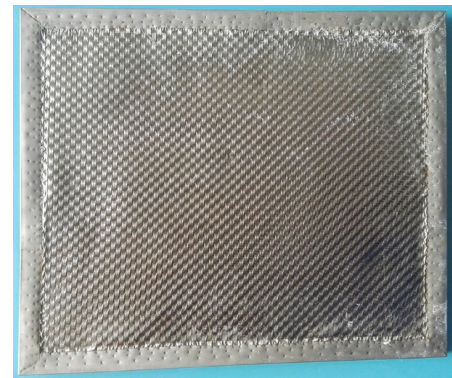
图 6 盐雾试验后焊接结构件宏观表面形貌 Fig.6 Surface morphology of welded structural parts after salt spray test
