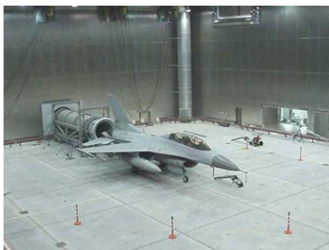
图 1 发动机尾气排放系统在韩国 ADD 环境室内的布置 Fig.1 Layout of the engine exhaust system in the ADD environment room in South Korea
