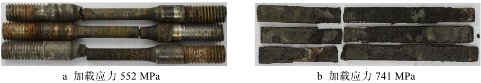
图 3 00Cr9-80 材质抗 SSC 实验后试样的宏观形貌 Fig.3 Macro morphology of the 00Cr9-80 sample after the anti-SSC experiment: (a) loading stress: 552 MPa; (b) loading stress: 741 MPa
