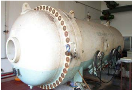
图 4 沈阳自动化研究所的卧式高压舱 Fig.4 Horizontal type high pressure simulator at Shenyang institute of automation
