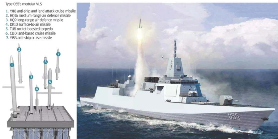
图 3 大型驱逐舰垂直发射装置模块分解图 Fig.3 The vertical launch device module decomposition structure of china large destroyer
