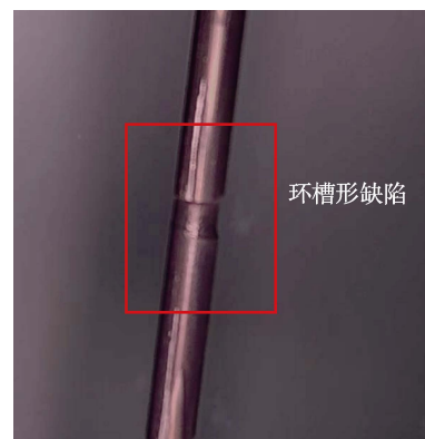
图 6 指套管在 P1 位置的磨损形貌 Fig.6 Wear profile of thimble tube at Point 1
