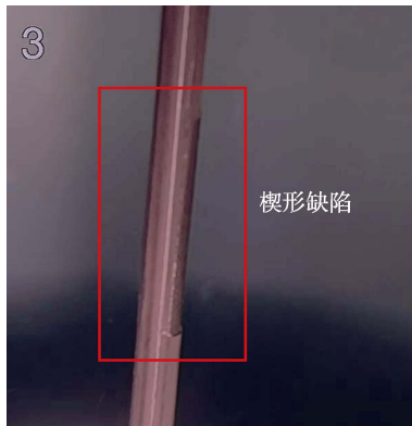
图 8 指套管在 P4 位置的磨损形貌 Fig.8 Wear profile of thimble tube at Point 4
