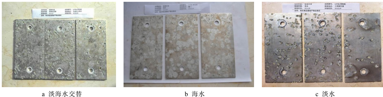
图 9 LF 6 M 带包铝淡水海水交替、海水和淡水自然环境暴露 2 a 腐蚀产物去除后的外观形貌 Fig.9 Appearance and morphology after corrosion products removed of LF 6 M clad aluminum in natural environments of freshwater-seawater alternating circumstance (a), seawater (b) and fresh water (c) for 2 years
