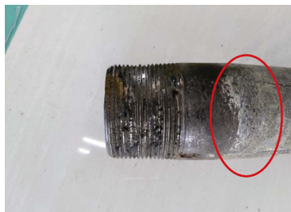
图2 失效件外壁形貌 Fig.2 Morphology of outer wall of failed parts
