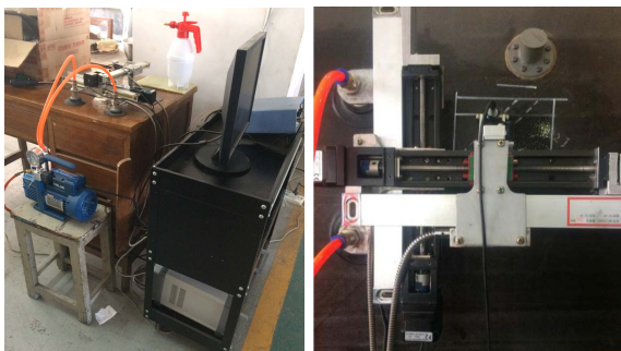
图 8 柔性自动特征扫描成像检测系统 Fig.8 Flexible automatic scanning and imaging nondestructive testing system (appearance and mechanism drawing)
