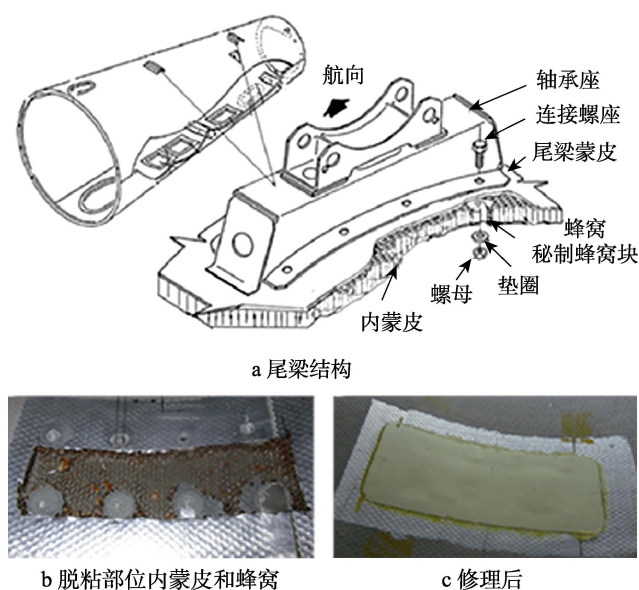
图 1 尾梁结构及修理前后脱粘部位内蒙皮和蜂窝 Fig.1 Tail beam structure (a) and inner skin and honeycomb of the deboned area (b) before and after repair (c)
