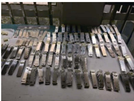
图6 经过拉伸剪切测试后的样品 Fig.6 Specimens after tensile shear tests
