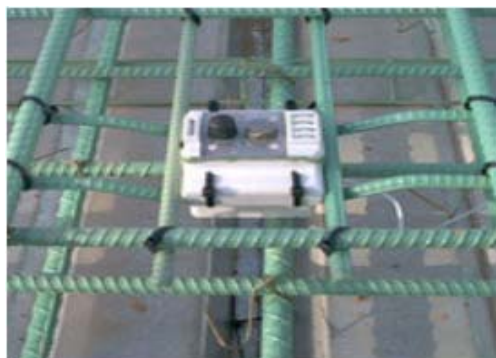
图6 工况下的嵌入式腐蚀监测传感器 [21] Fig.6 ECI sensor during operation [21]
