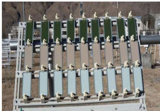
图 1 涂层试验样品户外暴露试验投试图 Fig.1 Outdoor exposure test of coating test sample
