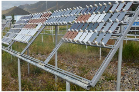
图 1 自然环境户外暴露试验 Fig.1 Outdoor exposure test in natural environment
