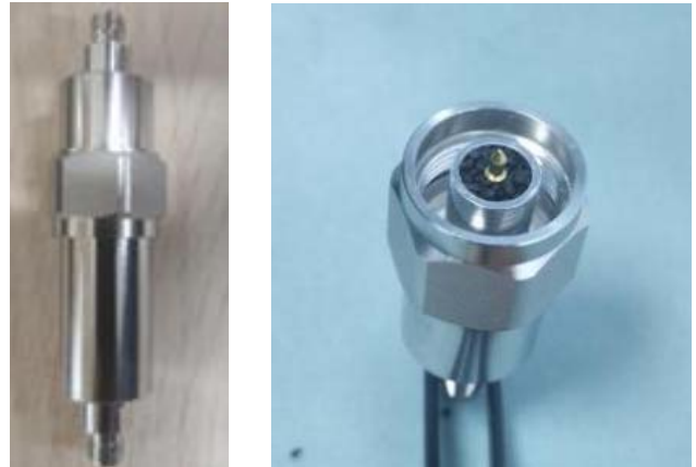
图 3 同轴夹具结构及火工药剂装填图 Fig.3 Structure of coaxial fixture and loading drawing of initiating explosives
