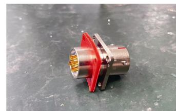
图 4 电连接器与制氧装置壳体搭接 Fig.4 Electrical connector connected to the oxygen generator
