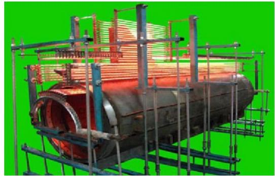
图6 轴向非分段加热方式试验示意图<sup>[68]</sup>Fig.6 Schematic diagram for axial non-segmented heating mode test<sup>[68]</sup>
