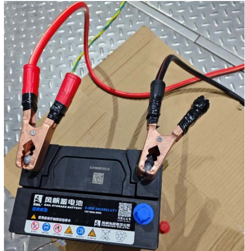
图 3 铅酸蓄电池恒流放电试验 Fig.3 Constant current discharge test of lead-acid battery
